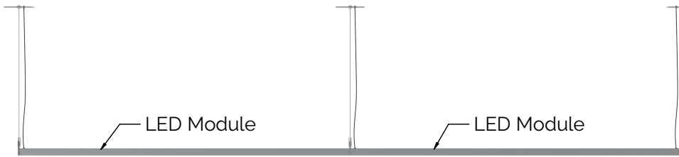
Two modules in continuous line
