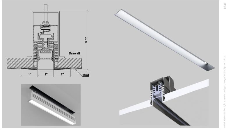
LeeSti Downlight is a recessed linear lighting fixture in 1', 2' and 4' lengths A cut off of 1' adds visual comfort to the space, the light source is not seen. Totally concealed in the architecture.
