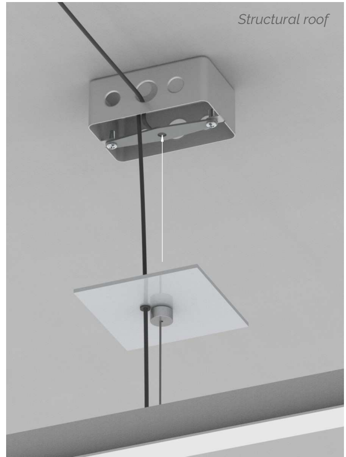
Step (6-8) : Securing fixture/Canopy to structural roof
